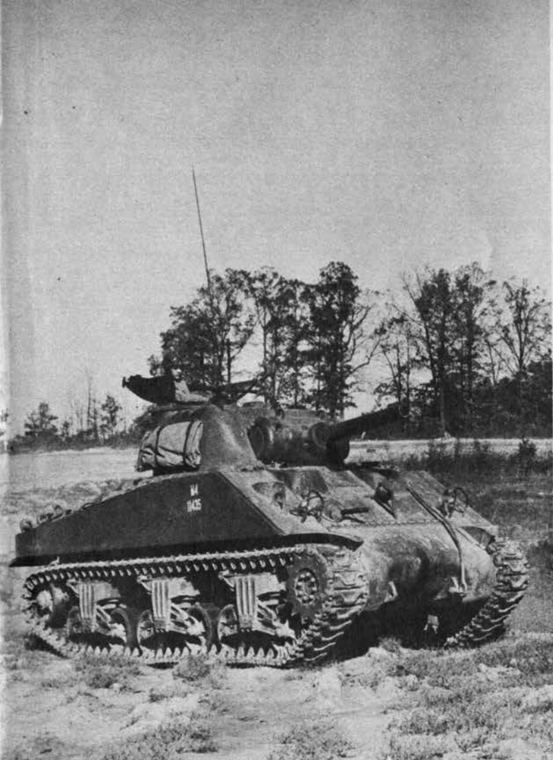
105-MM. HOWITZER ON M-4 HAS A SHORT BARREL, REINFORCED TURRET
